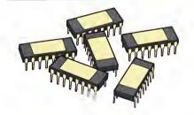
Main System Memory Expansion with the MEM Kit/16 provides additional 384 kilobytes of dynamic memory, upgrading standard 128K system to 512K in sockets already provided on mother board.
